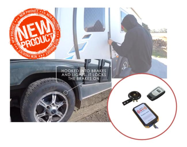
WiTi includes a revolutionary anti-theft system and is the only anti-theft system designed specifically for caravans and trailers fitted with electric brakes. If a caravan / trailer is hitched or moved slightly whilst the anti-theft is active then WiTi immediately applies the brakes, flashes all the lights and sounds an alarm.
