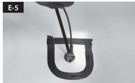
Insert Receiver & 5c Power cable through the hole
