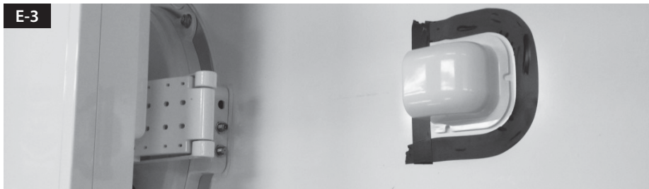
Arrange cable holder in front of (30cm apart from) antenna center by facing open side of cable holder toward projected part of the mounting plate. Then attach friction tape outside of cable holder
