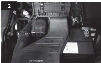
Check the Polarity of Car Battery (+/-)
